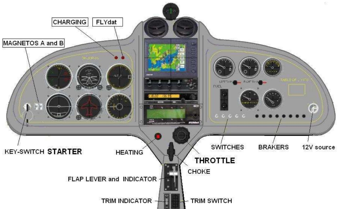
Fig.:Example of panel included standard analog instruments
