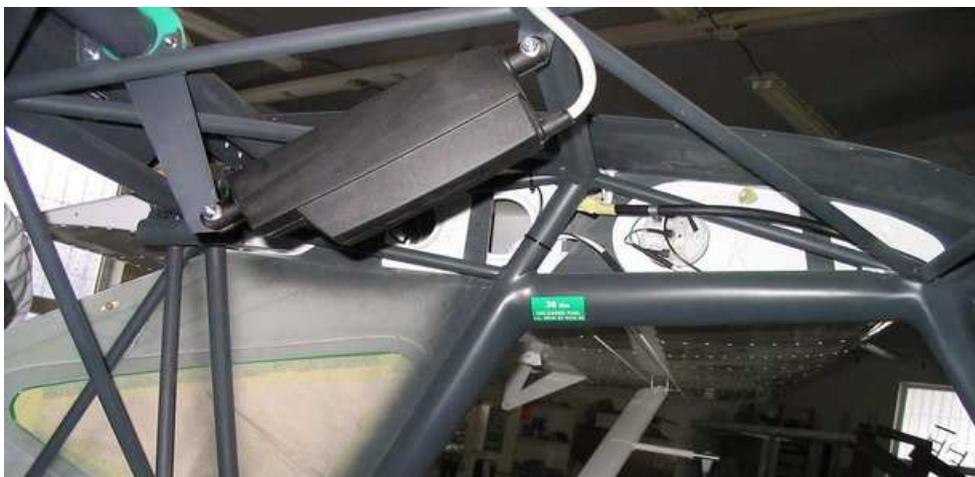
Fig.:Electric flap actuator
