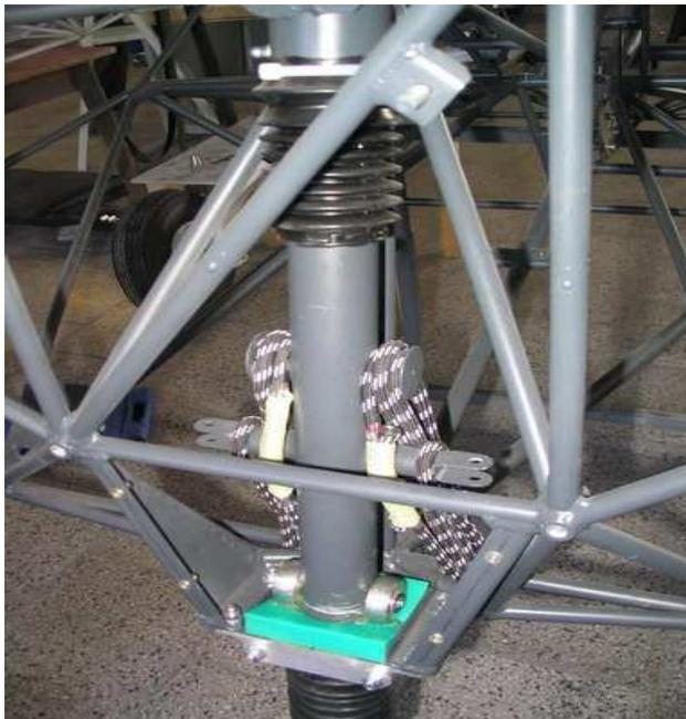
Fig.:Rubber cable suspension unit
