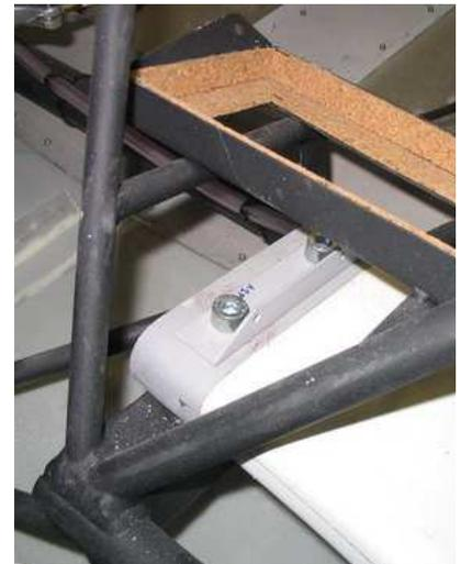
Fig.: Fixing of the main landing gear leg
