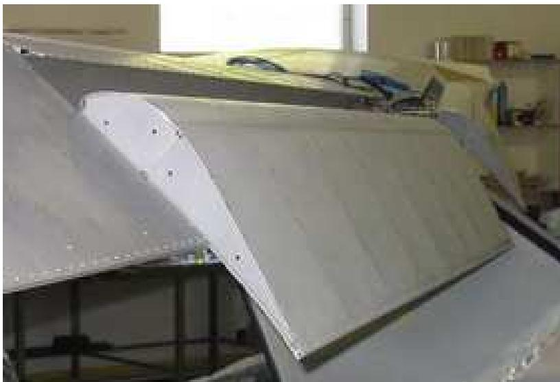
Fig.: Flaps in landing position
