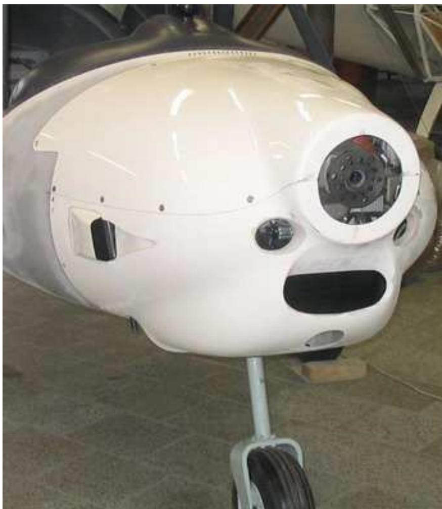
Fig.: Engine cowlings
