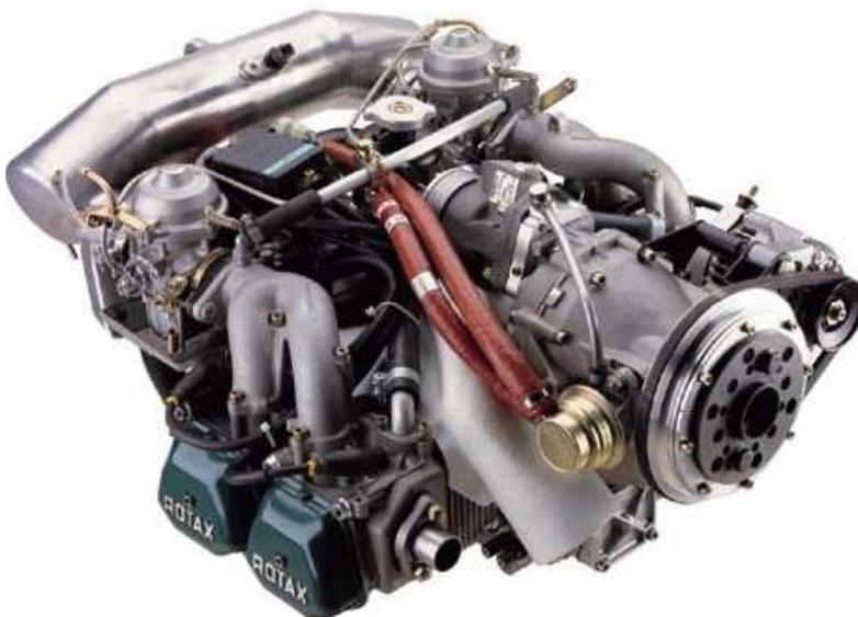
picture shows 912 ULS 3 -DCDI with options, alternator, airbox
