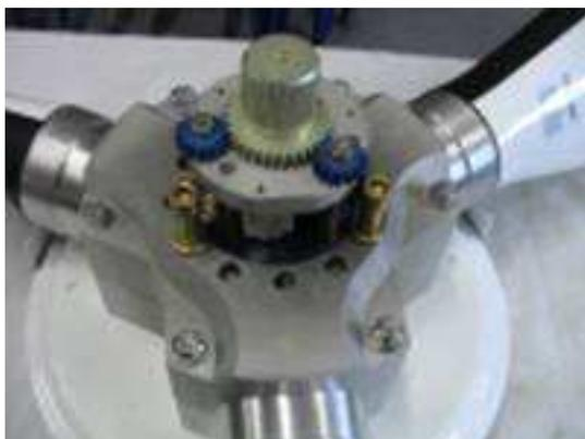
**The propeller SR 200** can be equipped with a central adjusting mechanism, which makes it possible to adjust all three propeller blades simultaneously, by means of a single control element. This ensures that all three propeller blades are permanently adjusted to the same working angle.
