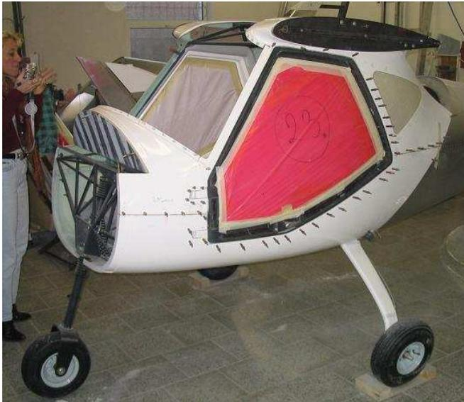
Cockpit fairing is produced from glass fiber composite, glued on the tubes and sheets of airframe and covers firewall, instrument panel including air vents, windshield frame in the front, connection to the wings in the top and door frames on the sides. In the rear COCKPIT FAIRING is equipped by foldable cargo compartment doors, needed to be folded for wing folding too.
