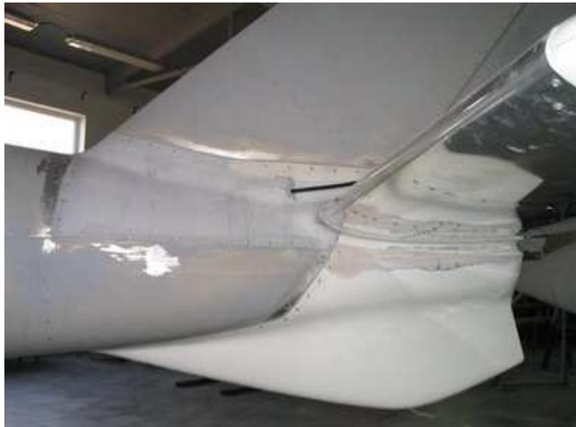
Fig.: Auxiliary tail skid
