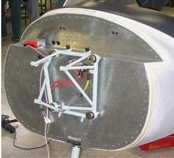
Fig.: Engine mounting
