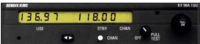
Bendix King KY97A transceiver (radio) - changeable with ICOM A200, good imunity oposite to interference
